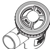
To speed up inhalation therapy, turn the speed selector (B2.2.3) clockwise.
