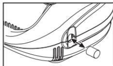
**To replace the filter, pull it out as shown in the figure.**
